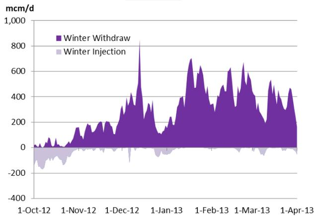
Figure 43 - UGS injection/withdraw profile. Source AGSI
