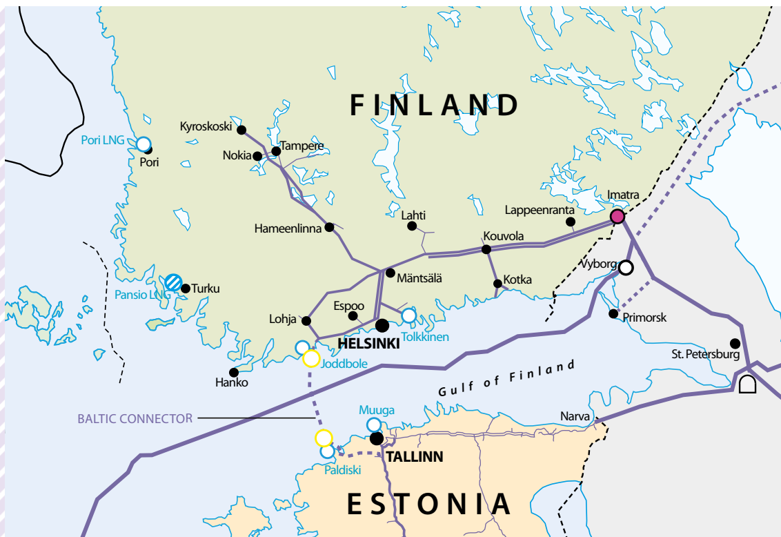
Figure 4.7: Natural gas transmission network, Finland
