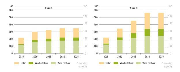
Figure 4.37: Installed generation capacities and share in the total generation capacity mix by source in Vision 1 and Vision 3
