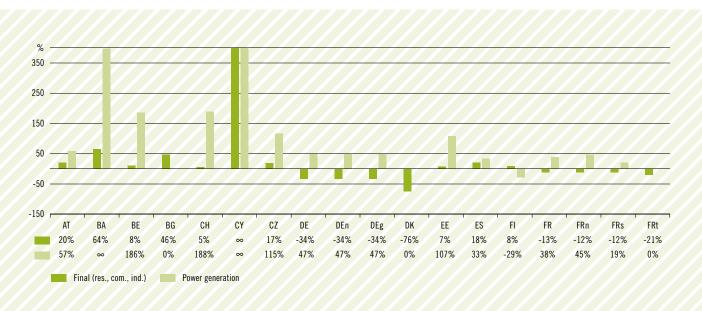
**Figure 4.29a:** GREEN: Evolution of total gas demand for the peak day in the period 2015 – 2035 per sector and balancing zone. Gas demand for power generation is based on data from ENTSO-E SO&AF 2014 – 2030 <sup>1)</sup>.
