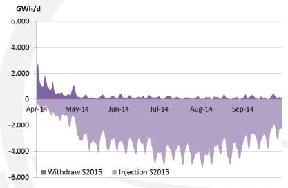
Figure 22 - UGS injection/withdraw profile EU-28 storages.
