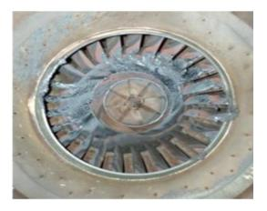
Flashback damage to burners has been linked to high levels of higher hydrocarbons
