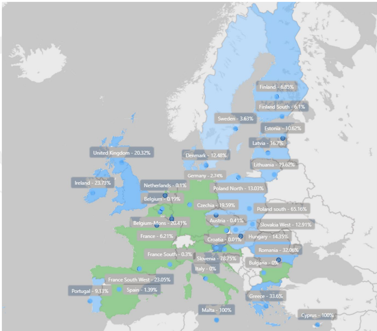
Figure 20: Yearly average hydrogen demand curtailment rate at country or node level in the advanced infrastructure level in 2030 for stressful weather year (unit: %).
