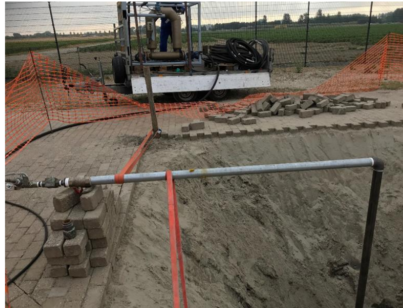
Nitrogen injection DN50 + Coriolis flowmeter
