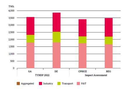
Final electricity demand is slightly higher (DE +10% and GA +5%) illustrating a deeper direct electrification
