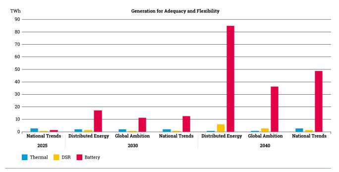
Figure 20: Peak generation, demand side response and battery technology (EU28)
