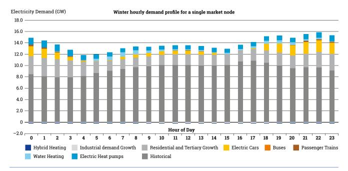
Figure 8: Example of winter hourly demand profile for a single market node – Impact of direct electrification in heating and transport sectors
