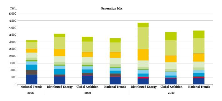
Figure 18: Electricity generation mix in Distributed Energy (EU28)
