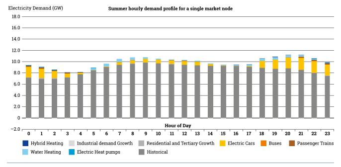
Figure 9: Example of summer hourly demand profile for a single market node – Impact of direct electrification in heating and transport sectors
