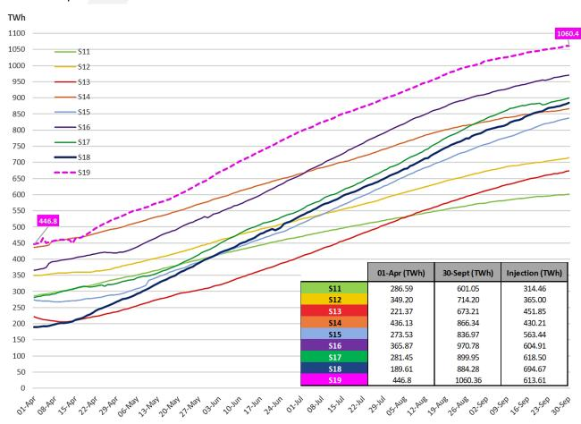
Figure 9.- Evolutions of UGS stock level. Summers 2011-2019 (TWh) (Source: AGSI+).
