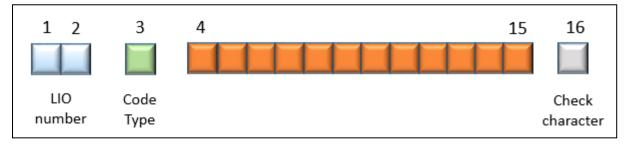
Figure 1 -Structure of an EIC code
