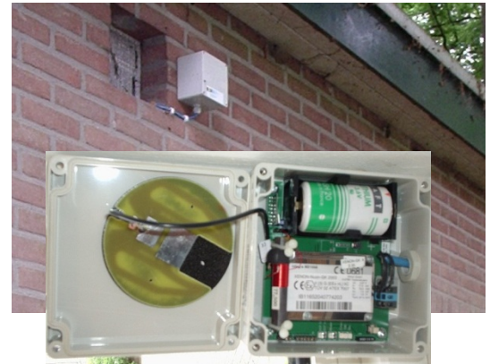
SMS battery modem: only used for daily metered connections
